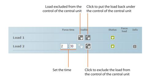
If the central unit detects that the set load limit is still being exceeded, the load in question will still be disabled.
