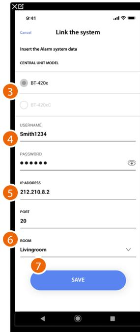
3. Select the type of control unit installed in the plant
