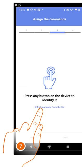
7. Press any one of the buttons on the command on the system
