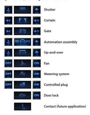
The group of icons formed by Curtain, Shutter, Gate, Up-and-over and Automation assembly must be used to control **two interlocked relays**; instead, the Fan, Controlled plug and Watering system icons control **single relays**, whereas the Door lock icon executes **Pushbutton**-type controls (PUL).
