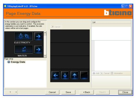
In the ITEM area there are the five objects available (ELECTRICITY, WATER, GAS, DHW (Domestic Hot Water), HEAT./COOL.) and CUSTOM. They can be used to configure the Consumption/Production Display system.
