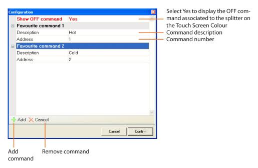
By dragging the "Group of commands" object to the Display area it will be possible customise its description. This command will be displayed on the Touch Screen Colour and will enable switching off all the splitters installed on the My Home system
