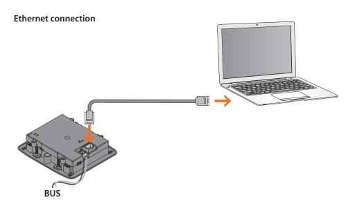
To ensure that communication is successful, Touch Screen must be on and it must be connected to the BUS.
