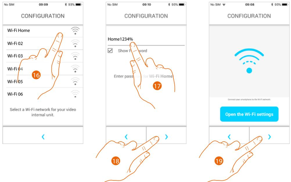
16. Now select the home Wi-Fi network to which the Connected Indoor Unit will be connected.
