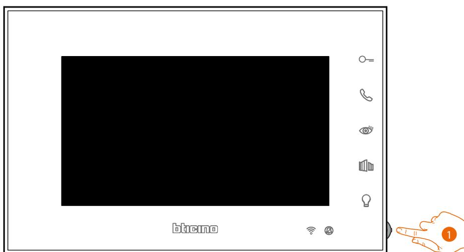
1. From stand-by press the joystick to activate the display.
