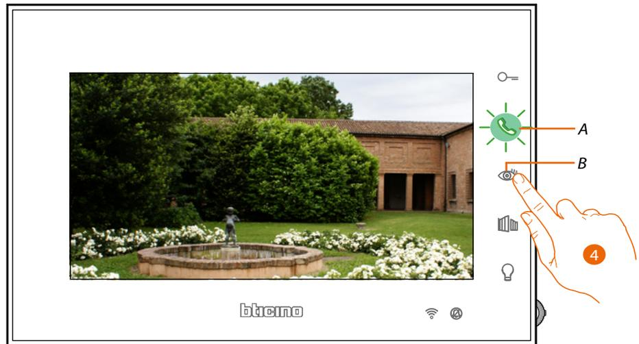
4. Touch to display another Entrance Panel or camera (using the scrolling service). When switching from one camera to the next the key (B) lights up. The (A) key flashes green; touch to enable communication.
