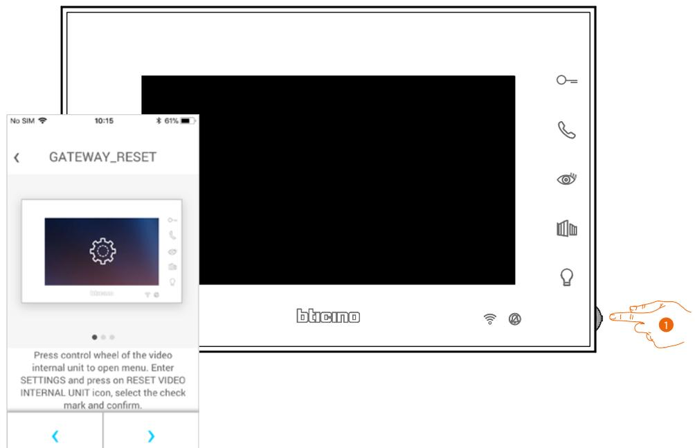
1. From stand-by press the joystick to activate the display.
