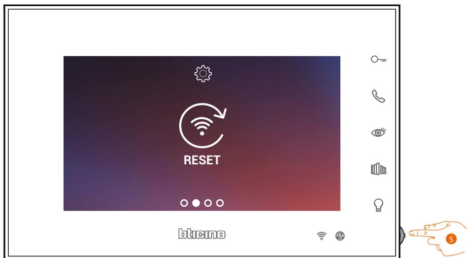
5. Press the Joystick to reset the Wi-Fi network and connect Connected Indoor Unit to another network, or to the same network with a different password.
