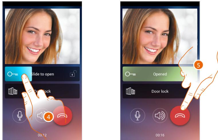
4. You can also open the door lock of the Entrance Panel from which the call comes, by dragging the switch. When it becomes green the door lock has been activated. If it remains blue, the command has not been performed correctly.
