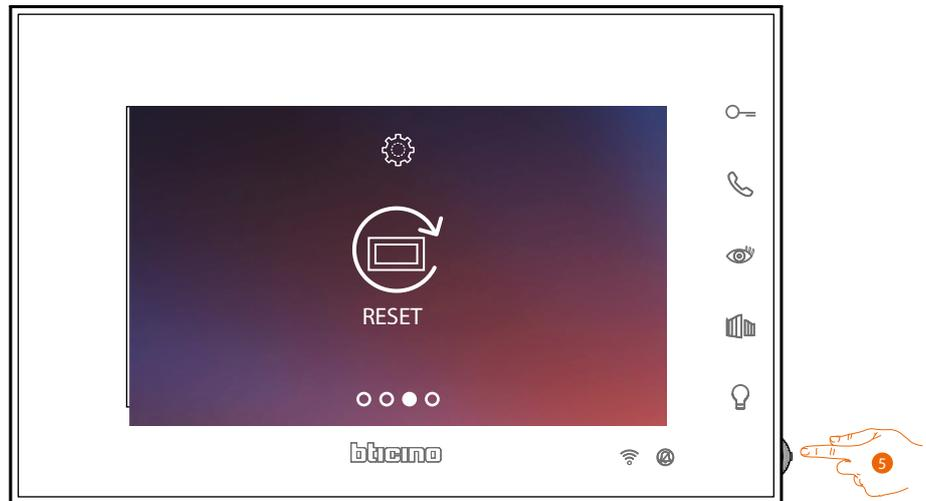
5. Press the joystick to reset the Connected Indoor Unit.
