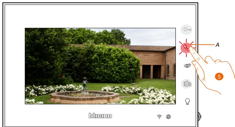
5. The key flashes red, touch to end the communication or wait for the automatic switch off time to elapse.
