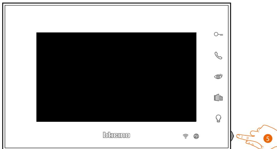
5. From stand-by press the joystick to activate the display.
