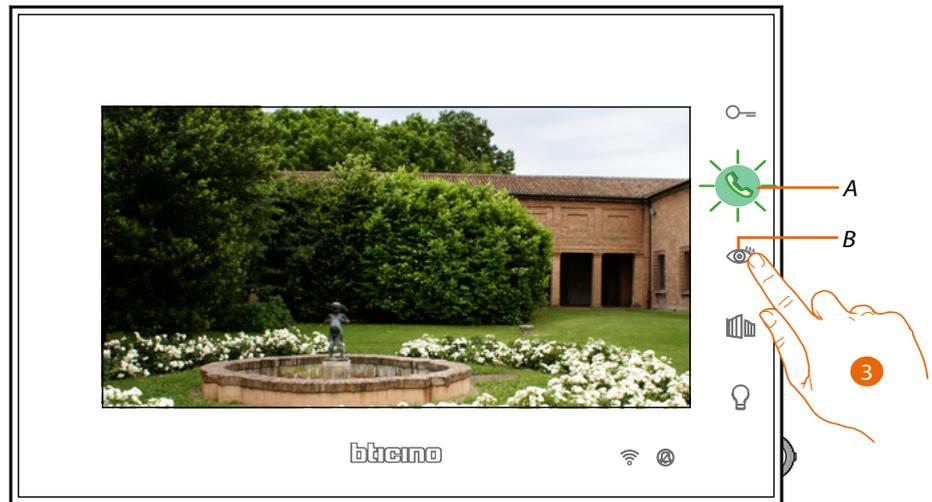
3. Touch to display another Entrance Panel or camera (using the scrolling service). When switching from one camera to the next the key (B) lights up. The (A) key flashes green; touch to enable communication.
