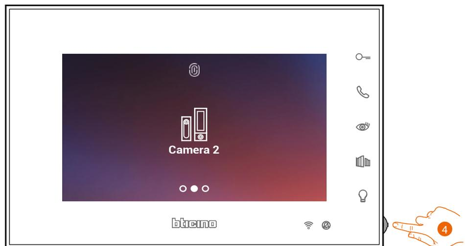
4. Touch to activate the desired camera, (the image is displayed for three minutes).
