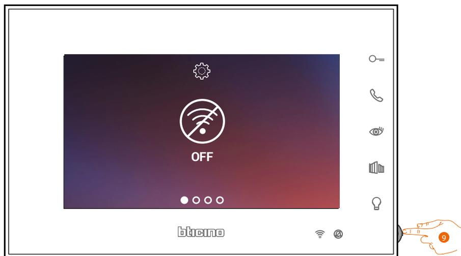
9. Touch to activate the temporary Wi-Fi network created by your Connected Indoor Unit. This screen appears, followed by a QR Code.
