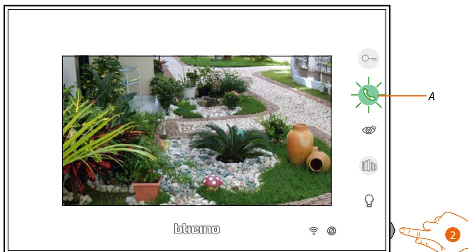
2. If necessary, during the call press the joystick to display the image sound/brightness/contrast/colour adjustment menu (see [Audio/video parameter adjustment](#))
