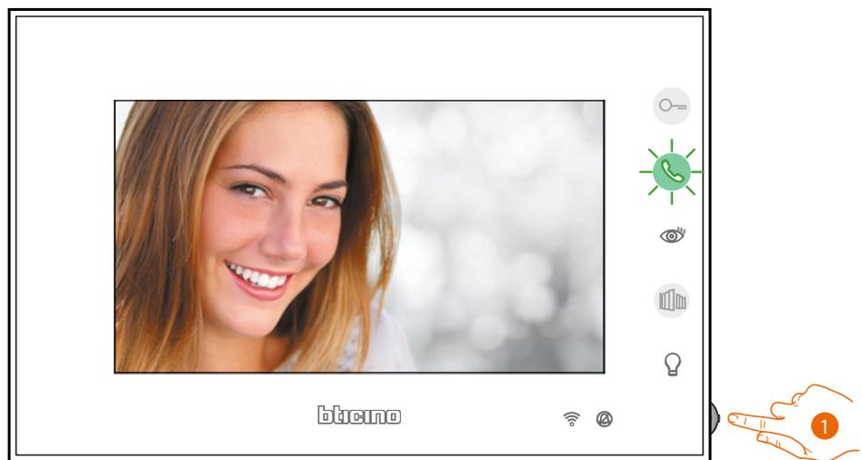
1. If necessary, during the call press the joystick to display the image sound/brightness/contrast/colour adjustment menu (see [Audio/video parameter adjustment](#)).
