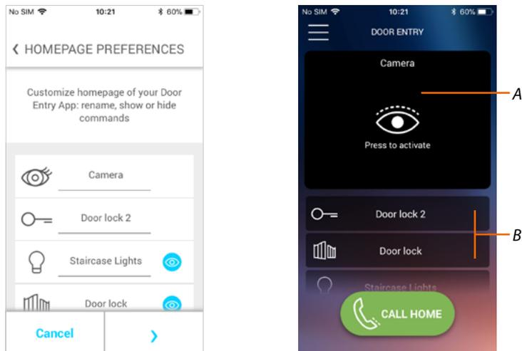
In addition to the staircase light key, the gate lock key can also be displayed in the Home Page. The Cameras/Entrance Panels will be available in the appropriate area (A), while for the door locks and staircase lights there is a dedicated key (B).
